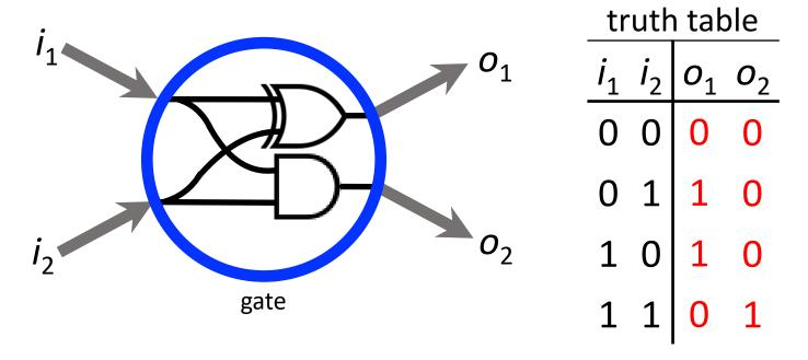
**gate:** function with two input bits  $i_1, i_2$  and two output bits  $o_1, o_2$
