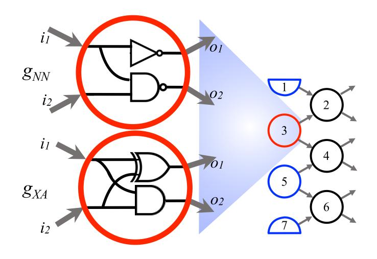
**Randomization**: Each row may be assigned  $\geq$  2 gates, with associated probabilities, e.g.,  $Pr[g_{NN}] = Pr[g_{XA}] = \frac{1}{2}$
