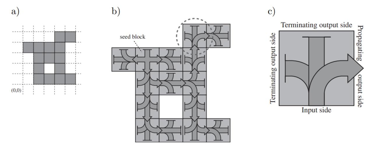
Fig. 5.1. Forming a shape out of blocks: (a) A coordinated shape S. (b) An assembly composed of  $c \times c$  blocks that grow according to transmitted instructions such that the shape of the final assembly is  $\tilde{S}$  (not drawn to scale). Arrows indicate information flow and order of assembly. The seed block and the circled growth block are schematically expanded in Figure 5.2. (c) The nomenclature describing the types of block sides.
