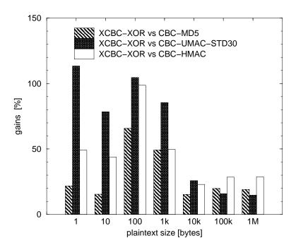
Figure 2: Percentage gains of the DES-XCBC\$-XOR mode over the CBC-MD5, CBC-UMAC-STD30, and CBC-HMAC-SHA1 modes for message sizes of 1 B – 1 MB.
