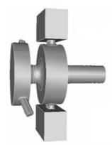
Figure 3. Omega3P model of the Linac Coherent Light Source radiofrequency cavity. Courtesy of the Advanced Computation Department, SLAC.
