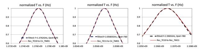
Fig. 3. Normalized transmission curves and the Lorentzian fit for the cavity modes at 1.176 GHz (left), 2.057 GHz (middle), and 2.196 GHz (right).
