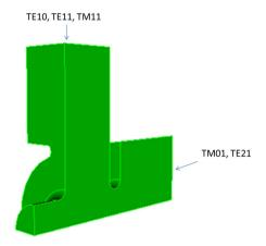
Fig. 1. A quarter model of a pillbox cavity coupled with rectangular waveguides and circular beampipes. The two symmetry planes are set to be magnetic boundary conditions. Three rectangular and two circular modes are loaded at the rectangular and downstream circular waveguides, respectively.
