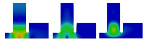
Fig. 2. Electric field amplitude profiles on the vertical symmetry plane for cavity modes at 1.176 GHz (left), 2.057 GHz (middle), and 2.196 GHz (right).
