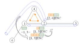
Figure 7 Packet looping by routing interference
