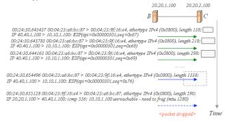
Figure 4 DETER lab emulation results of example 2
