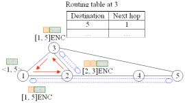
Figure 8 Packet looping considered as IP spoofing
