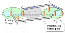
Figure 1 Tunnel Overlap due to routing interference
