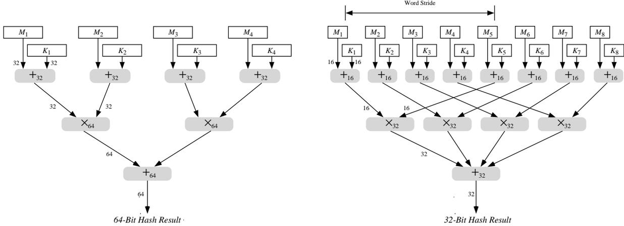
Figure 2: **Left:** The NH hash function in its “basic” form, using a wordsize of  $w = 32$  bits. This type of hashing underlies UMAC-STD-30 and UMAC-STD-60. **Right:** The “strided” form of NH, using a wordsize of  $w = 16$  bits. This type of hashing underlies UMAC-MMX-30 and UMAC-MMX-60.
