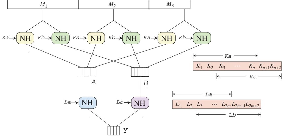
Figure 4: The T2 scheme. Each block of the message is hashed twice, first using a key  $Ka$ , and then using a key  $Kb$ . Key  $Kb$  is the shift of key  $Ka$ . The outputs of the  $Ka$ -hashes are concatenated and  $La$  hashed, and the outputs of the  $Kb$ -hashes are concatenated and then  $Lb$  hashed. Key  $Lb$  is once again the shift of key  $La$ .
