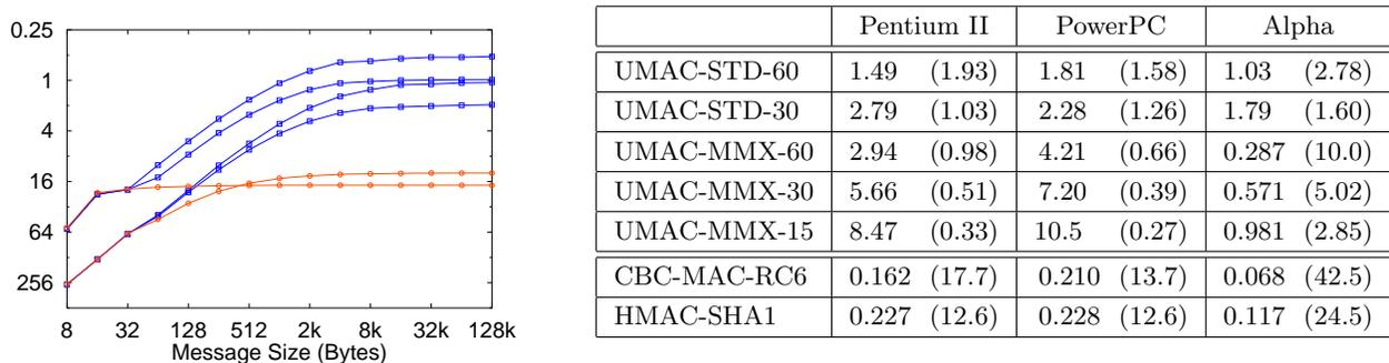
Figure 3: UMAC Performance. **Left:** Performance over various message lengths on a Pentium II, measured in machine cycles/byte. The lines in the graph correspond to the following MACs (beginning at the top-right and moving downward): UMAC-MMX-30, UMAC-MMX-60, UMAC-STD-30, UMAC-STD-60, HMAC-SHA1 and CBC-MAC-RC6. **Right:** Peak performance for three architectures measured in Gbits/sec (cycles/byte). The Gbits/sec numbers are normalized to 350 MHz.
