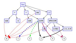
Fig. 5: The coiled AST for the idiom in Figure 6-8. The colors and line effects differentiate the arrows to references for readability.
