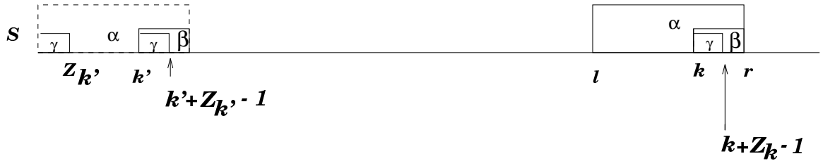
Figure 3: Case 2a. The longest string starting at k' that matches a prefix of S is shorter than |\beta| . In this case, Z_k = Z_{k'} .
