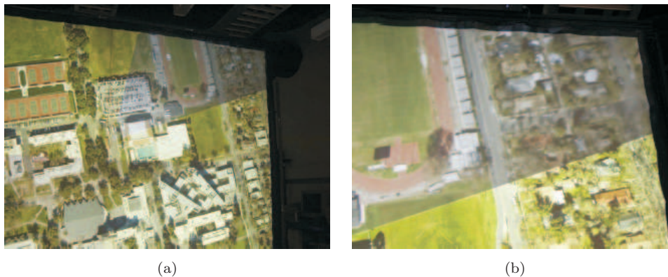
Fig. 11. (a) The inset is moved to the top-right corner of the display wall and is partially cut off. (b) Even though the calibration produces satisfactory results, the close-up view reveals that the effective resolution of the foveal inset projection has dropped below the resolution of the display wall. A projector with longer throw distance can be used to solve this problem.
