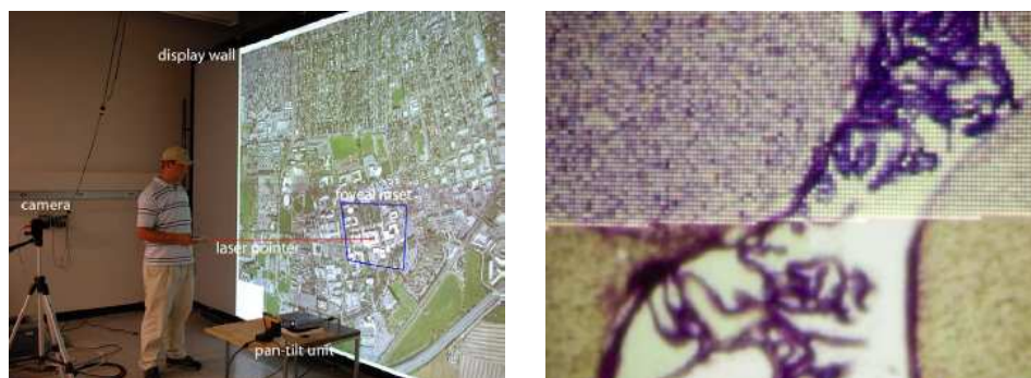
(a) The user directs the projection of the foveal inset using a laser pointer. The size of the projected inset is significantly smaller than the tiles of the rear-projected display wall, thus providing a higher resolution.
