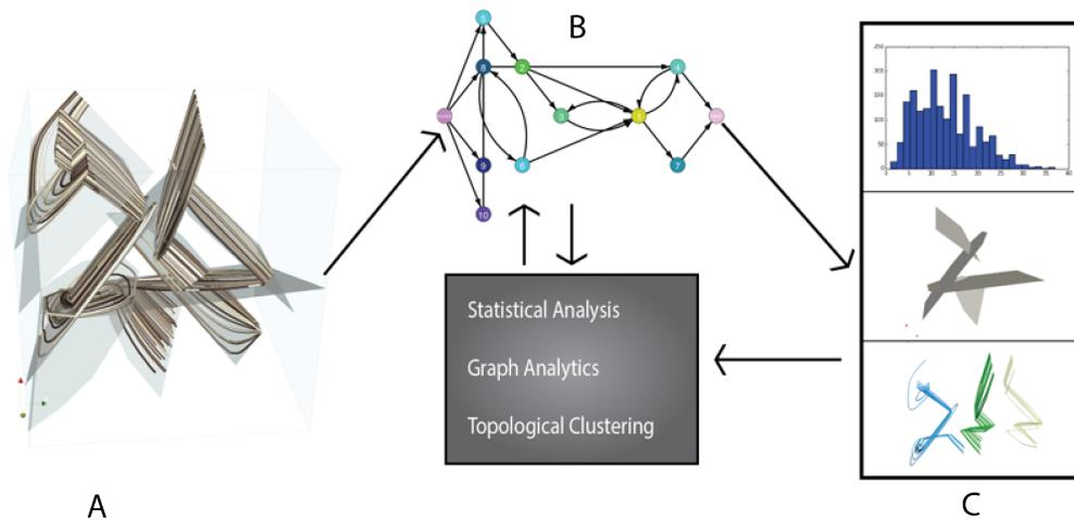
Figure 4 To automate flow and transport analysis for discrete fracture networks (A), we use a graph representation (B) from which we extract statistical properties, paths of concentrated flow and clustered particle traces (C). This method allows us to automate analysis of large numbers of flow simulations and store them in a database for use with DORA. (Image courtesy of Aldrich et al.<sup>12</sup>)
