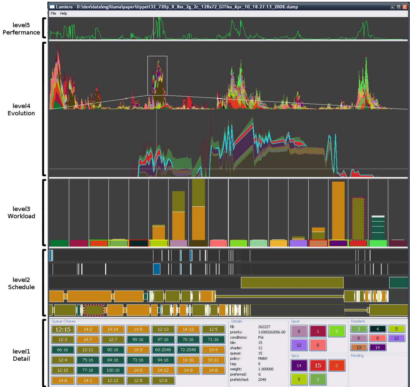
Figure 2: The stack of widgets of the Lumière tool. The layout and interconnection of the widgets allow users to drill down to problem spots in the execution. At the top, Performance and Evolution views provide much needed context and coarse-grained viewing of a derived performance measure contrasting it with the actual workload distribution over the referenced static data. The Workload view breaks down this workload for a specific scheduling decision into its individual tasks. The scheduled tasks are shown in the Schedule view below, arranged in time lines for each execution unit and the raw measured details are presented in the bottom most Detail view. The multiple views of the synchronized state across the various layouts provide the basis for Lumière's effectiveness.
