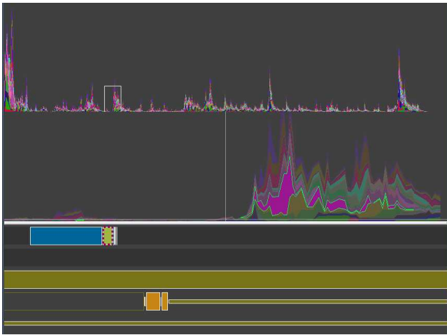
Figure 4: Evolution and Schedule views when using windows to dispatch pixel computation tasks. Schedule view, from top to bottom: two CPUs, one reader and two GPUs. Before each “spike” the dispatcher kernel is executed (light-colored box with the dark, dashed outline in the first CPU’s timeline).
