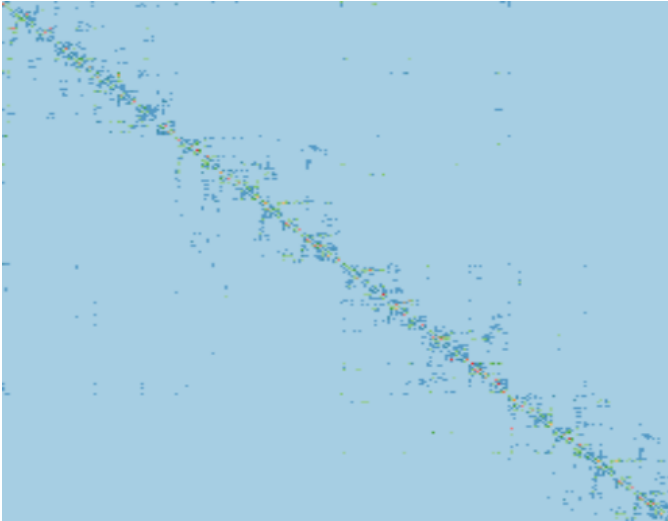
Fig. 5. Communication matrix of 256 processes during the load balancing phase of SAMRAI, color mapped by the number of bytes exchanged.
