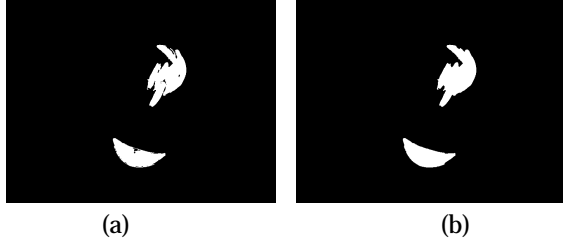
Fig. 9. Post-segmentation: (a) result of the region growing process for a particular image; (b) binary image representing the final segmentation, after applying the rolling ball.
