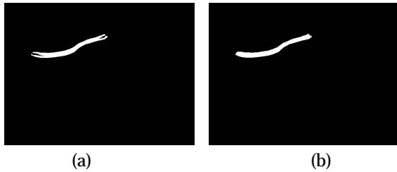
Fig. 10. Rolling ball: (a) binary image resulting from the region growth process; (b) result obtained by the rolling ball.
