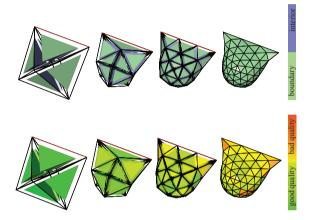
**Figure 8:** Three steps of the subdivision scheme with preservation of a sharp crease (red edge). The upper row shows the exploded view of the mesh. The lower row visualizes the quality of the tetrahedra measured with the minimum dihedral angle criterion from red (bad quality,  $0^\circ$ ) to green (good quality,  $\approx 71^\circ$ ).
