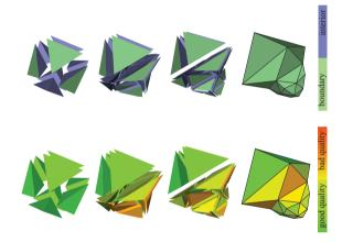
Figure 10: Two subdivision steps with adaptive refinement. Here, the interpolating boundary scheme was used.
