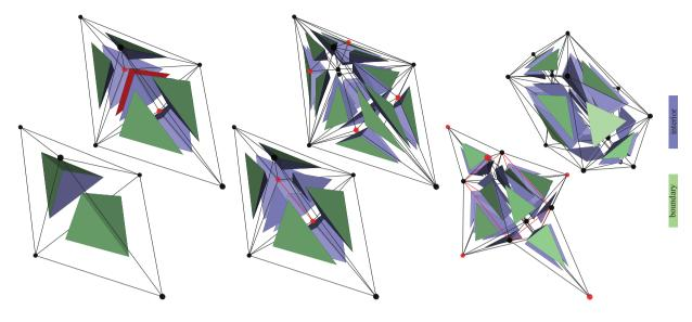
Figure 1: An example for our tetrahedral subdivision scheme. Starting from the input mesh (bottom left) we show from left to right: the mesh after 1-4 splits, 2-3 face flips, boundary 1-3 splits, boundary edge flips, edge removals and geometric smoothing.
