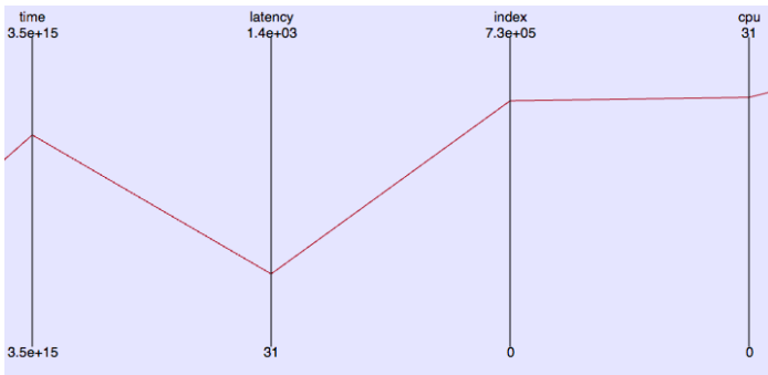
Fig. 3: The parallel coordinate visualization for a single memory access sample. The red line represents the sample, and the black lines represent its attributes. The intersections denote the values of the sample for each attribute.
