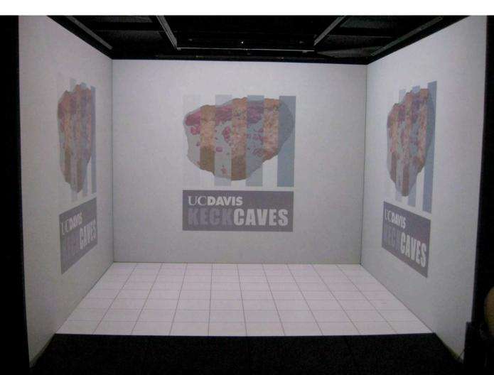
The KeckCAVES: A user perceives a seamless three-dimensional environment that can be explored by manipulating data within the 800 ft<sup>3</sup> space
