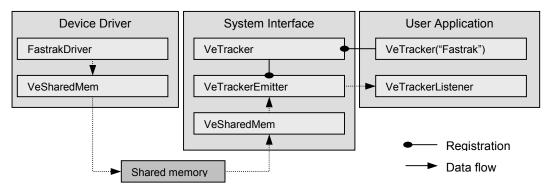
Figure 5: Example of device abstraction layer and message passing.
