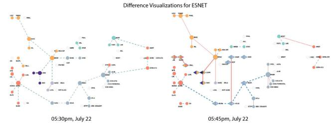
**Fig. 4** Flow changes between 05:15 pm–05:30 pm, July 22, and 05:30 pm–05:45 pm, July 22. Large node size indicates large flow change. Dashed blue lines show reduction in network flow, and red
