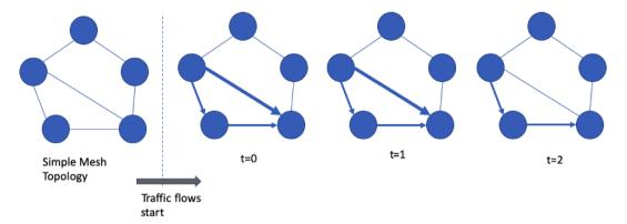
(A) Simple network mesh topology shown with traffic flows at times t=0,1 and 2. The thickness of the edges represents the amount of traffic flowing between nodes.
