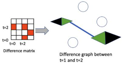
(C) Difference graph between adjacent time steps, caused by addition or deletion of an edge. The left half of the rhombus represents the community of the node for time step  $G_t$  and right half for time step  $G_{t+1}$ . The sizes of the nodes depict the magnitude of change.
