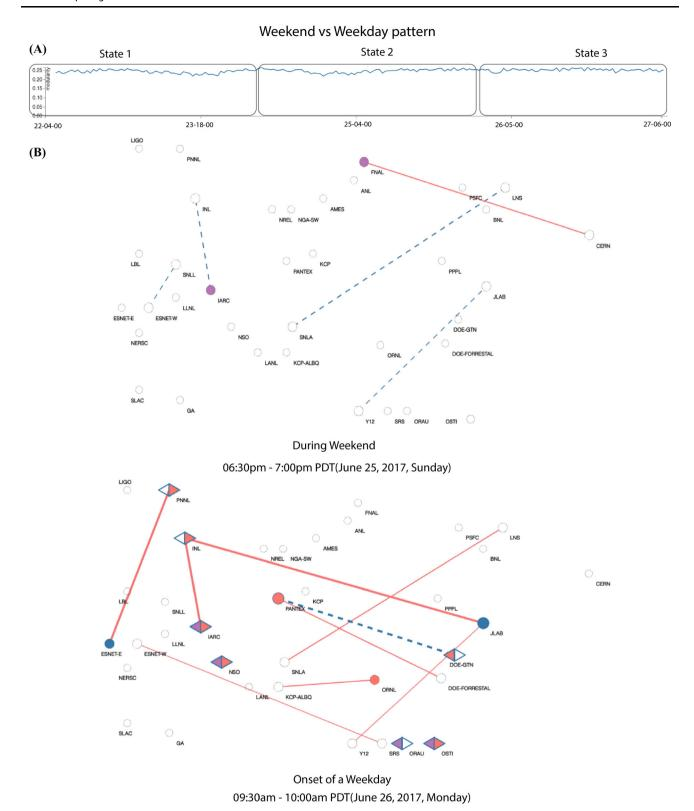
**Fig. 7** Metrics plots and difference topology of network flow in ESNeT network over a larger time window. **A** Evolution of modularity metric for period *June 22, 4.00 am–June 27, 6.00 am PDT*. The method detects three major states pertaining to weekend and weekday temporal states; **B** Difference graphs, during weekend state (top) and state change from Sunday to Monday, weekend to
