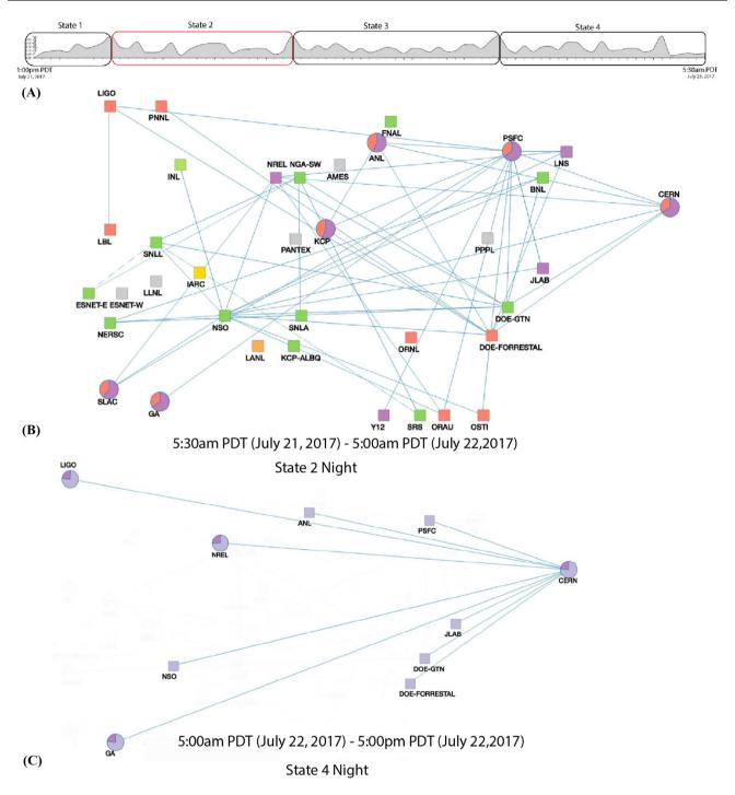
**Fig. 5** Similarity and difference plots for ESNet flow. **A** Plot of similarity metric showing four states, indicating day/night patterns. **B** Similarity visualization for period from 21 July, 5:30 pm, to 22
