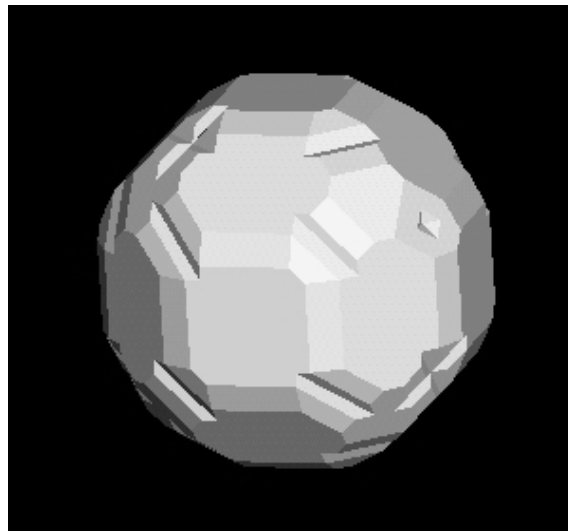
Figure 6. Approximation of spherical isosurface based on approximately 36,000 center leaf points.
