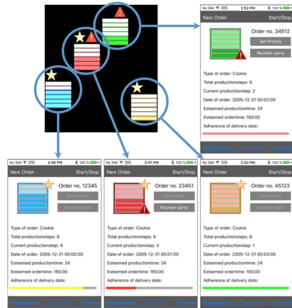
Fig. 13 Touch input applied to the status update view on the smart watch opens a dedicated status report view on the smart phone.
