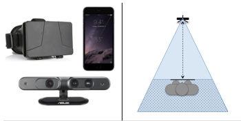
Figure 3: 3D camera setup: Asus Xtion Pro Live 3D camera and VR viewer fixing iPhone 6Plus (left). Viewing angle of camera limits user's movement ability (right).
