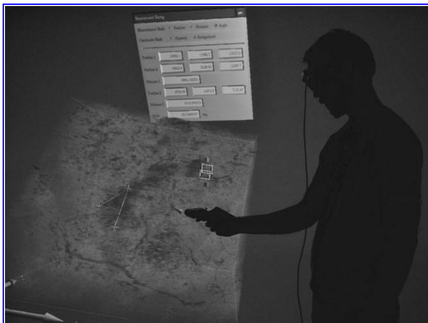
FIG. 4. A user analyzing the fenestrate microbialite sample in the CAVE. The Measurement Dialog window is in the background. The cube between the user and volume represents a cutting plane assigned to a Virtual Input Device; it remains fixed in space. Three white points connected by lines within the sample represent the Measurement Tool markers. They are placed on a surface representing a support with ORZ in the three-dimensional volume.
