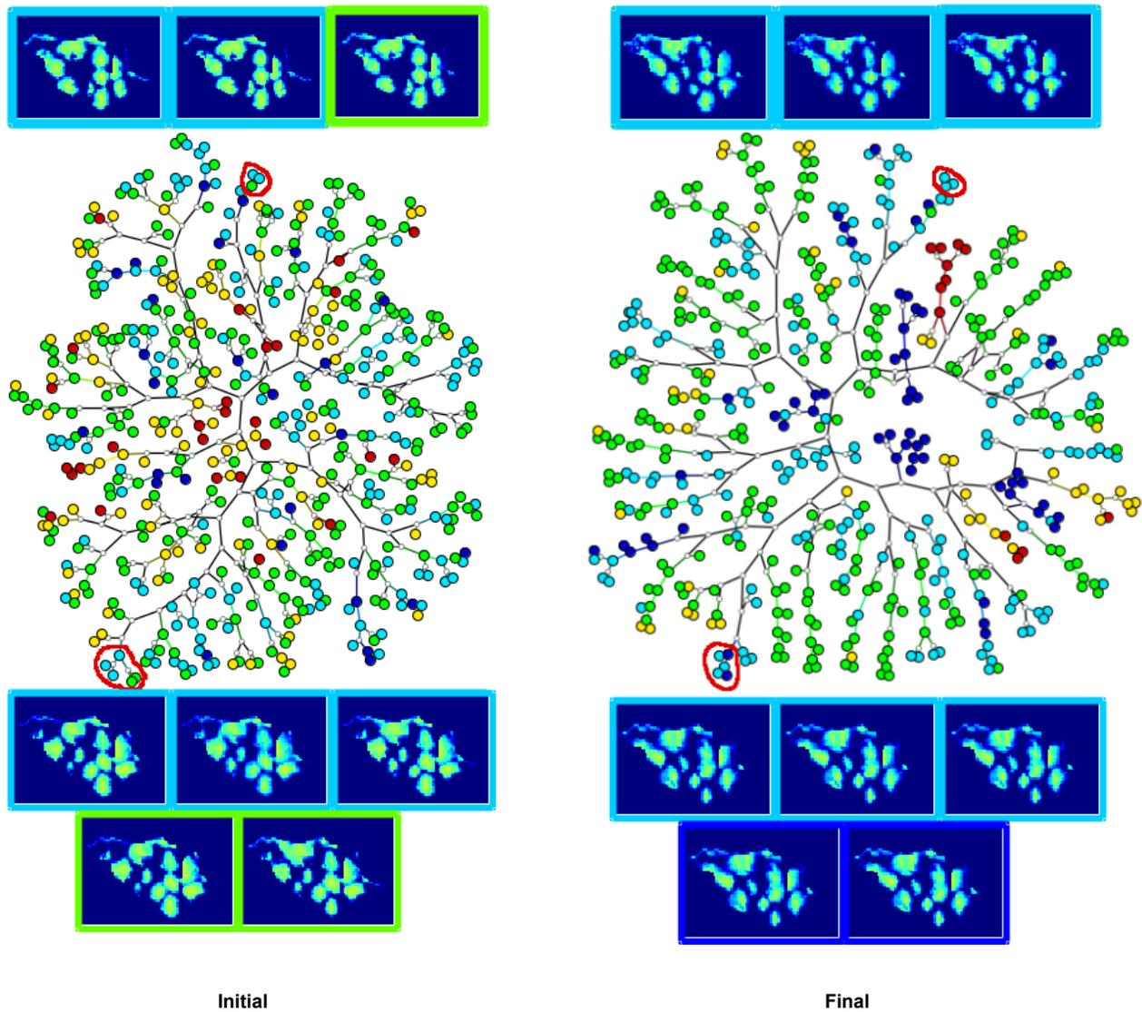
Fig. 6— Visual variability analysis of 500 simulation models from two data-assimilation iterations (initial on the left, final on the right). The global quality matching is defined as the number of OFs that present errors inside the cutoff value  $[-5,5]$ . Detailed views of some branches of two data-assimilation iterations. Each model is represented by a colored circle.
