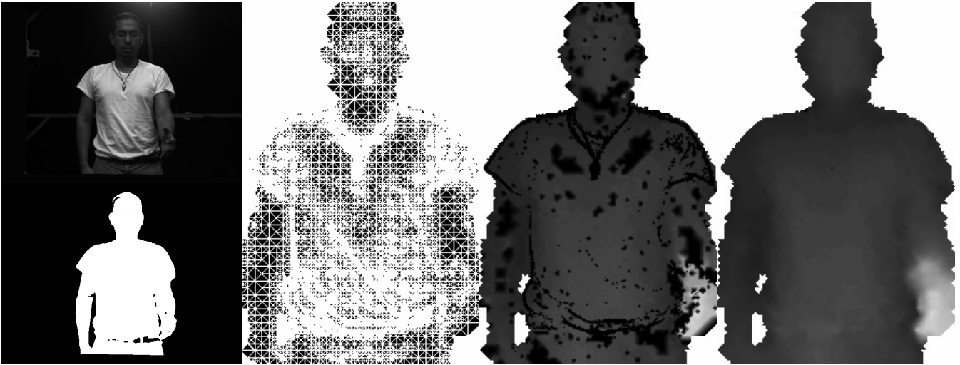
Figure 8: A 320 \times 240 image taken from a single camera in a stereo cluster (top-left), a background subtracted image generated for that image (bottom-left), the mesh generated for this image (second image from the left), the pre-processed disparity image (third image from the left), and the post-processed disparity image (right image). Note that lighter gray values indicate that the object in the scene is closer, darker gray indicate that an object in the scene is further away, and black indicates areas of uncertainty.
