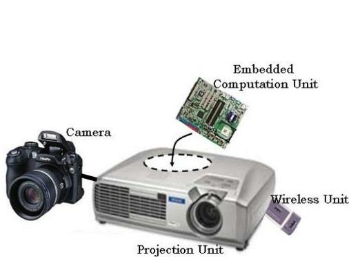
Figure 1: A Plug-and-Play Projector (PPP) consisting of a camera, a projector, and a processing unit.
