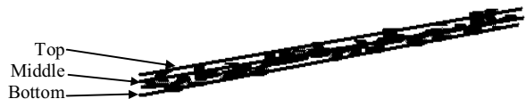
Figure 7. Last line of Figure 6 with the three estimated straight lines at top, bottom, and middle using least square method
