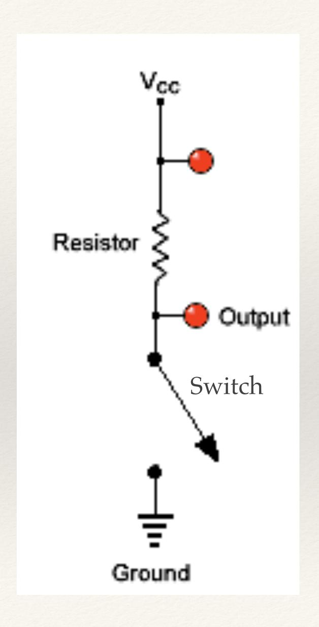
If switch is off (0) (equivalent to the presence of the block)
