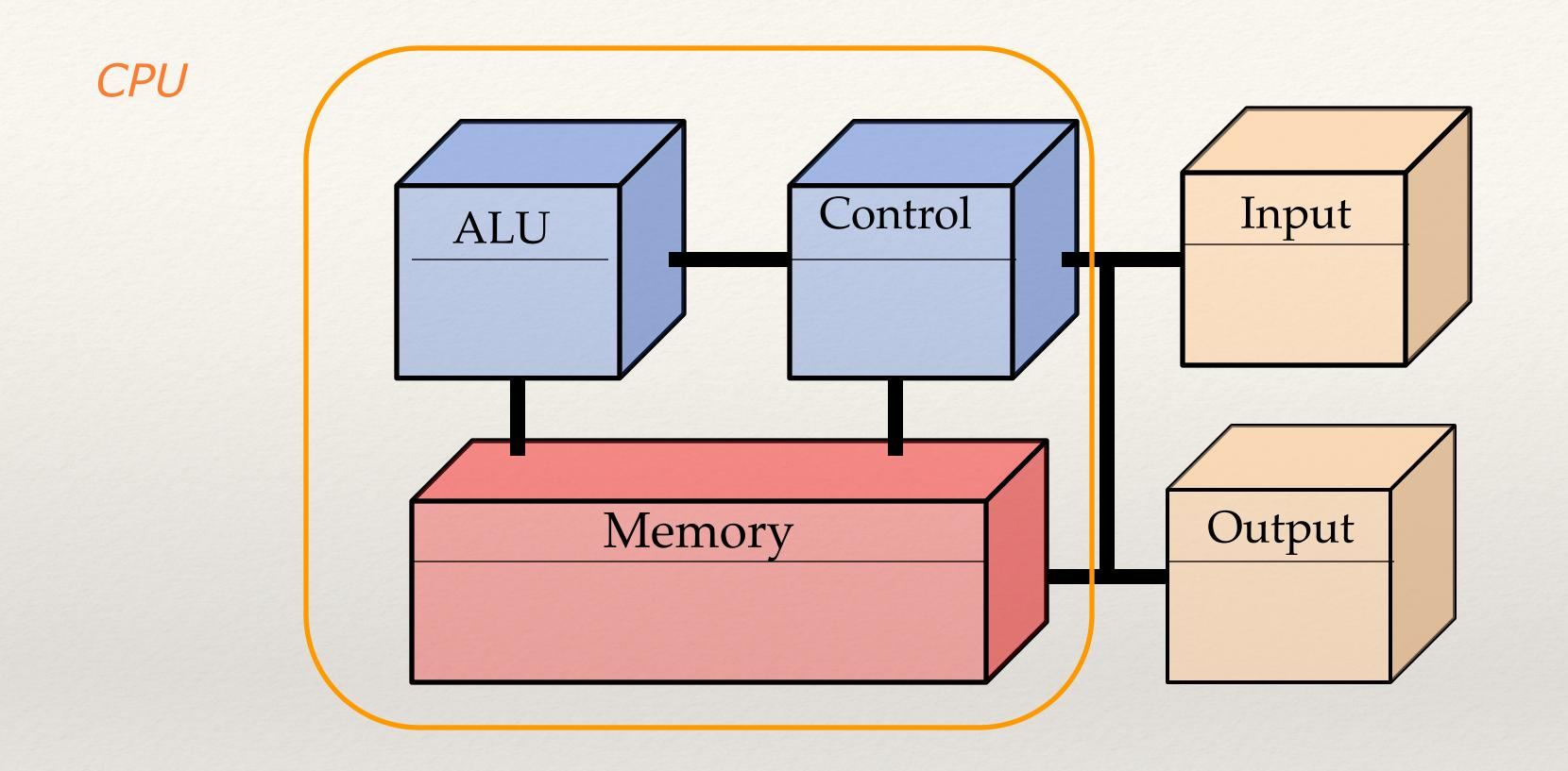
The CPU consists of three parts: the Arithmetic Logic Unit (ALU) The Control Unit Memory
