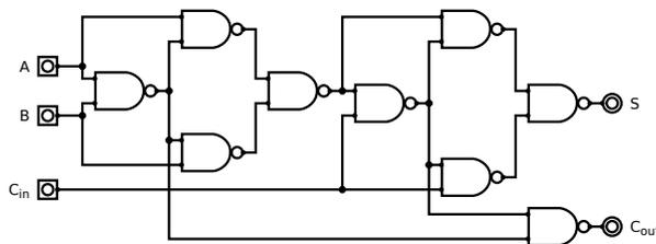
Does WFA compute the desired functions  $s$  and  $c'$ ? (Treat labels  $A$ ,  $B$ ,  $C_{in}$ ,  $S$ , and  $C_{out}$  as synonyms for  $a$ ,  $b$ ,  $c$ ,  $s$ , and  $c'$ ). Explain how you made your determination.
