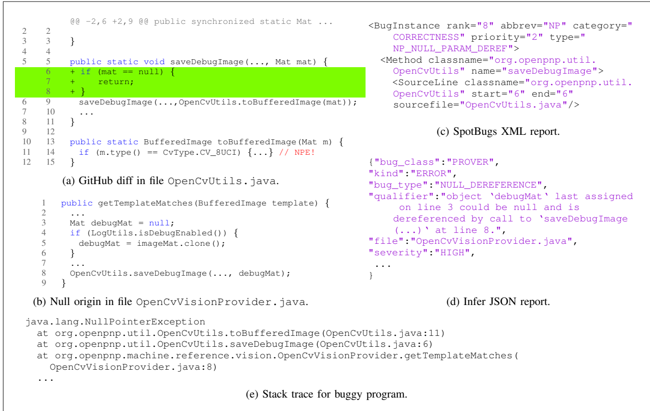
Fig. 2: GitHub diff, stack trace, SpotBugs XML report, and Infer JSON report for an NPE found by SPOTBUGSLT and INFER.
