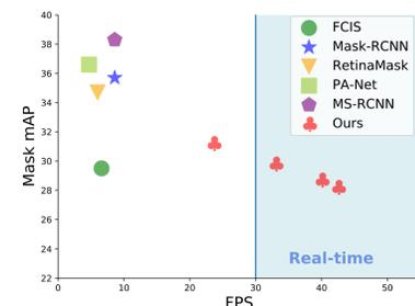
**YOLACT** [1] is the first *real-time* (above 30 FPS) instance segmentation approach with competitive instance segmentation accuracy on the challenging MS COCO dataset.
