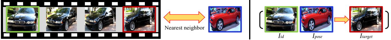
Figure 3. Constructing ID, pose, and target training triplets. With this procedure, we automatically obtain supervision to train our model.
