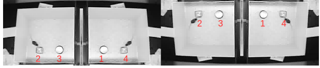
Figure 4. Data augmentation via horizontal/vertical flipping and 180-degree rotation. From left to right: original frame, vertical flipping, horizontal flipping, and 180-degree rotation. We update the labels accordingly.
