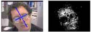
Figure 7: Orientation of the flesh probability distribution marked on the source video image
