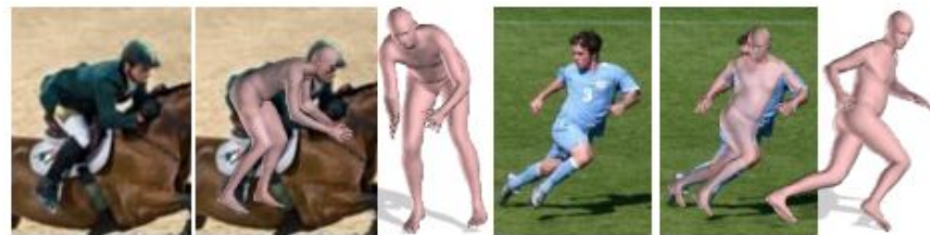
Fig. 1. Example results. 3D pose and shape estimated by our method for two images from the Leeds Sports Pose Dataset [22]. We show the original image (left), our fitted model (middle), and the 3D model rendered from a different viewpoint (right).
