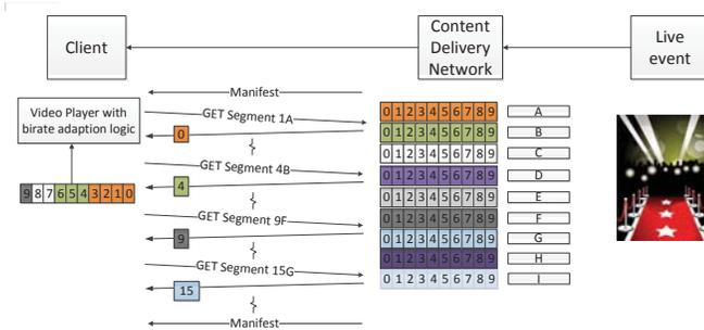
Fig. 1. Architecture of adaptive video streaming for a large-scale live event
