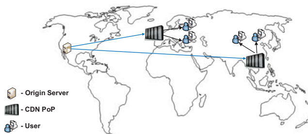
Fig. 1. Architecture of a Content Delivery Network (CDN)
